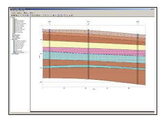
The WinFence cross-section module of GaeaSynergy can be used to quickly create detailed full-color cross-sections. A wide variety of strata can be used to create cross-sections. Types of strata that can be used include layers, faults, lenses, intrusions, mineralization, contamination, and hydrocarbons.
